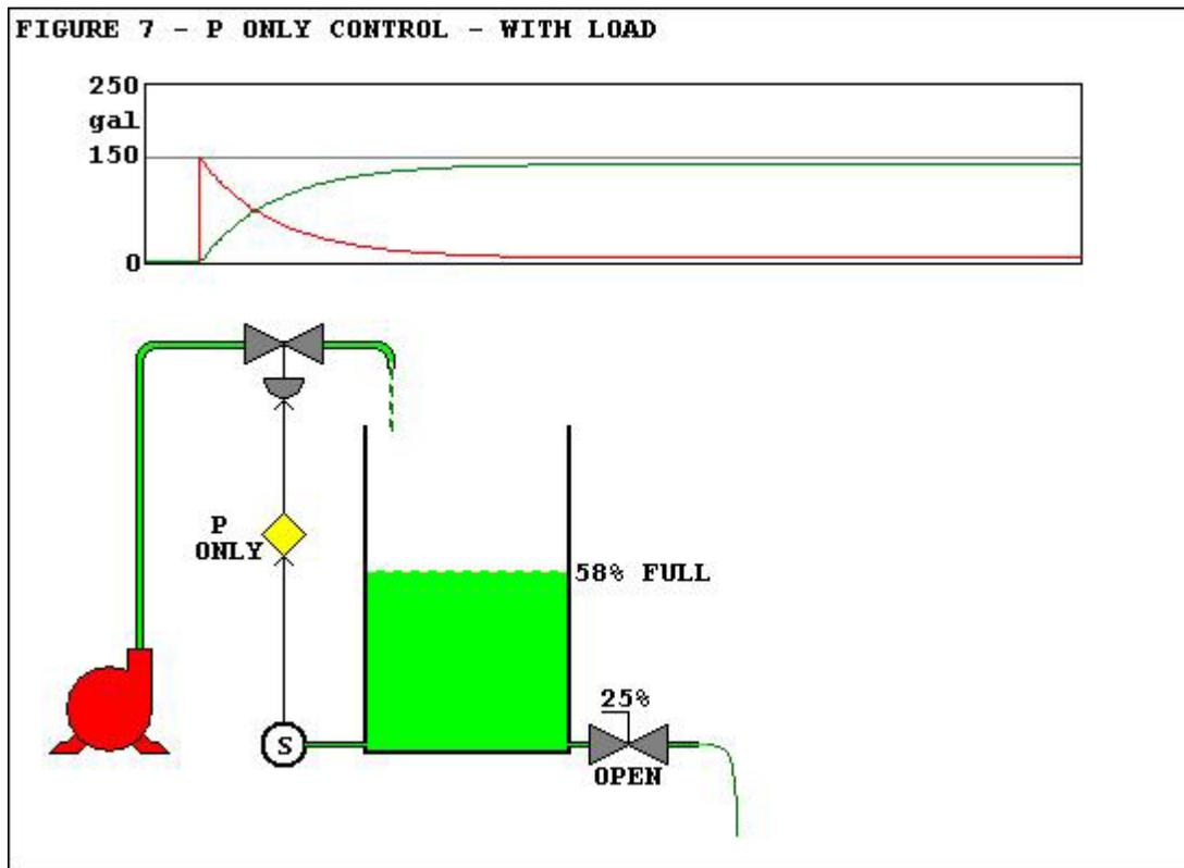
so now we no longer have a "sealed system" ... the "load" represented by the water draining away from the tank produces the classic "droop" or position slightly below the setpoint that we normally associate with a Proportional-only controller ... and so instead of the 60% target which we desire, something more along the lines of about 58% is the best that our Proportional-only controller is able to give us ...
