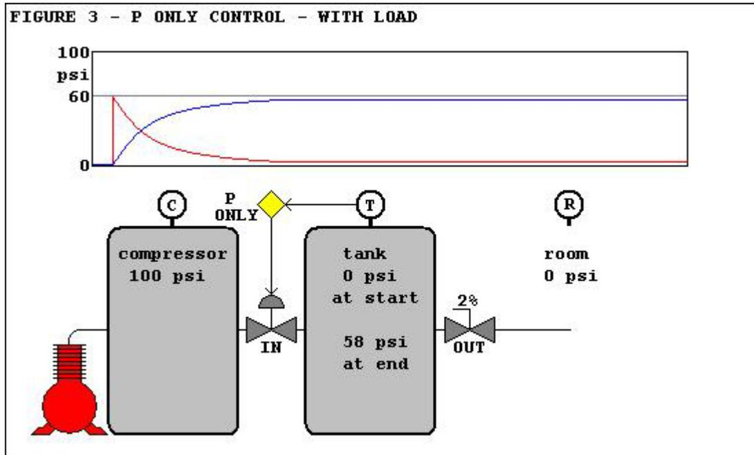
notice that in this example, the pressure never gets quite all the way up to the setpoint ... instead it settles out at some slightly lower pressure and then continues along that path ... this is the same type of "steady state" situation that we had with the oven example in my earlier article ...
