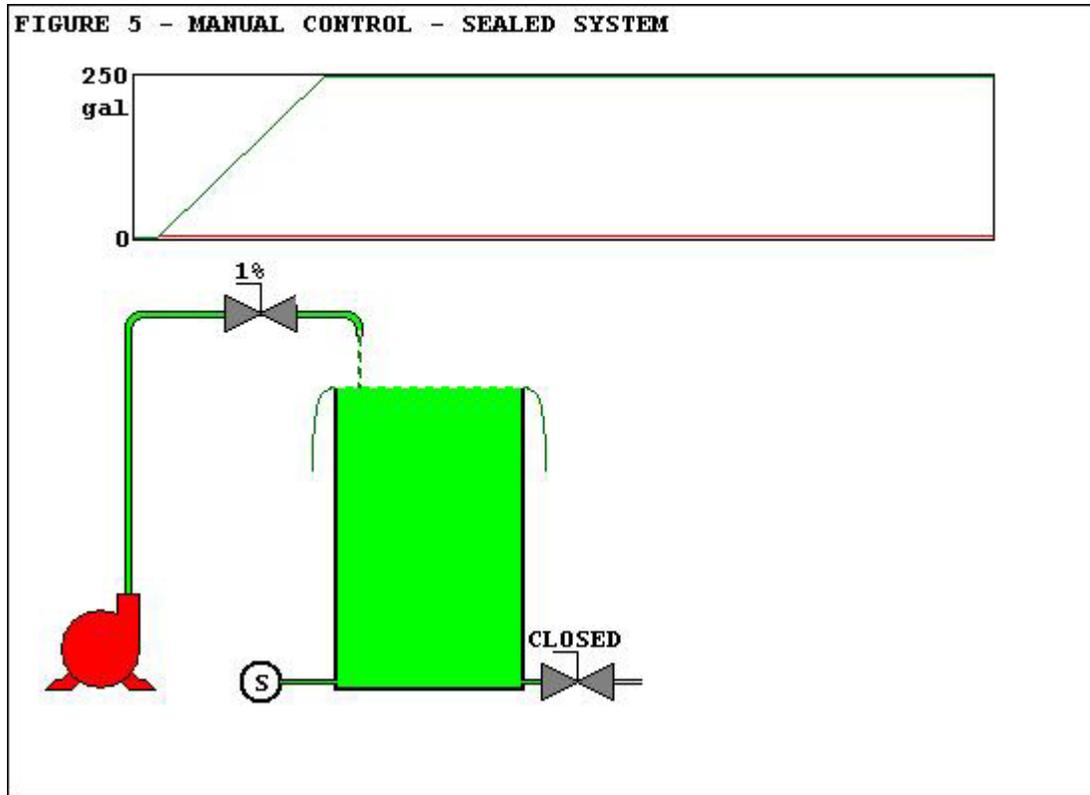
now keep in mind that the tank we're using for our example is a straight-sided vessel and that we're maintaining a constant rate of fill ... but under these conditions, basic common sense and life's experiences are enough to convince us that, sooner or later, the tank will become full and then overflow ...
